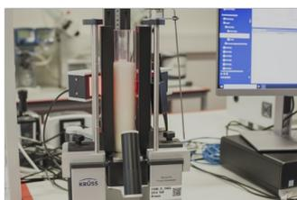
Fig.1 : Krüss Foam analyzer with drink sample
